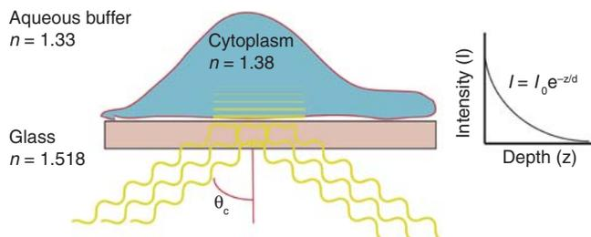
**FIGURE 1.** Total internal reflection. The angle of the incident light above the critical angle is totally internally reflected back from the coverslip surface. The reflected beam generates an evanescent field that decays exponentially into the sample. TIR illuminates molecules near ( $\sim 100$  nm) the glass surface. In live cell imaging, TIR only excites molecules in or near the cell membrane and significantly reduces background fluorescence.
